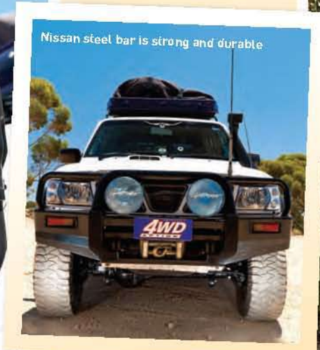
Snorkel and Unifilter keep the air dry and clean
